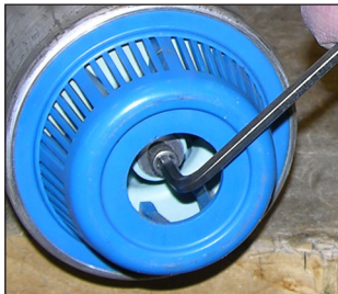
Figure 2: Turn Wrench to Rotate the Pump Shaft
