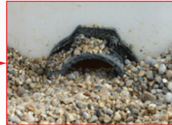
Pipe failure with seal and fitting contamination
