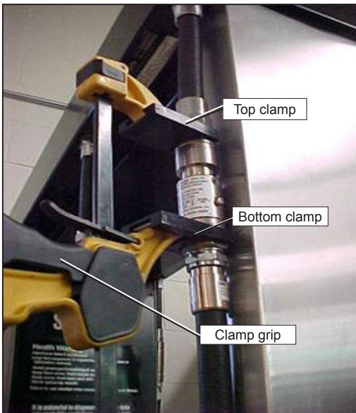
Figure 9: Breakaway Clamp Installed
