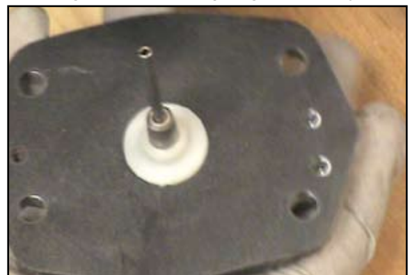
Figure 4: Diaphragm Installed in Cover
