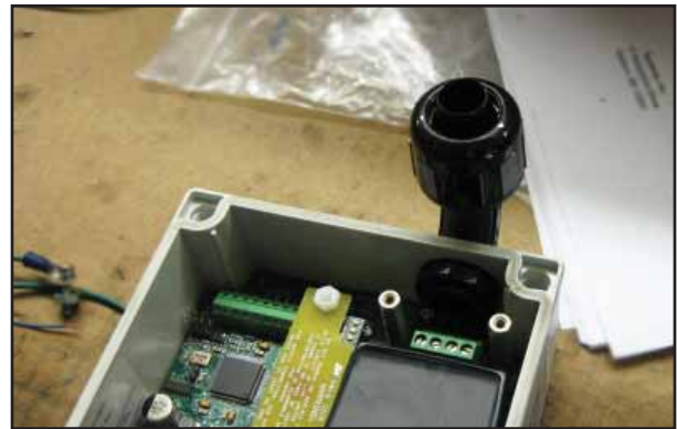
Figure 8: 90-Degree Fitting Installed
