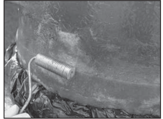
Figure 10 - Removing Air Bubbles
