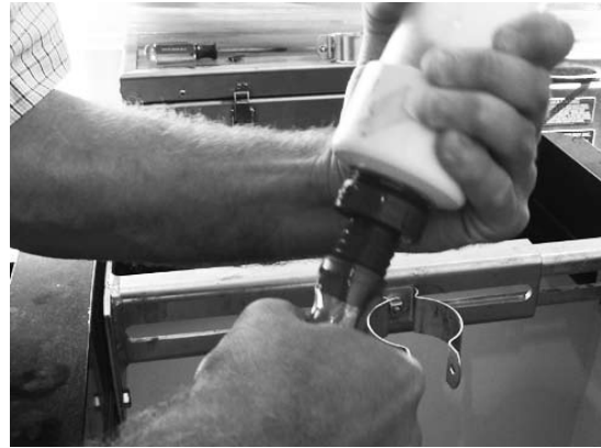
Figure 42 - Installing Sensor Housing to Hose
