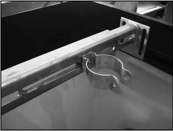
Figure 40 - Sensor Clamp on Stabilizer Bar
