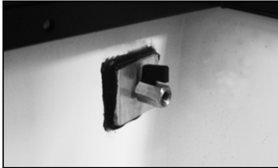
Figure 44- Vacuum Port in Open Position
