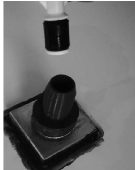
Figure 38 - Removing Plug from Port
