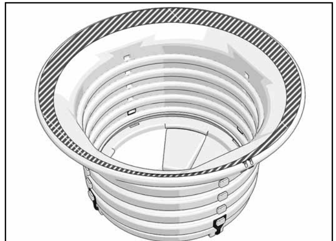
Figure 12: Clean Weld Area on Riser
