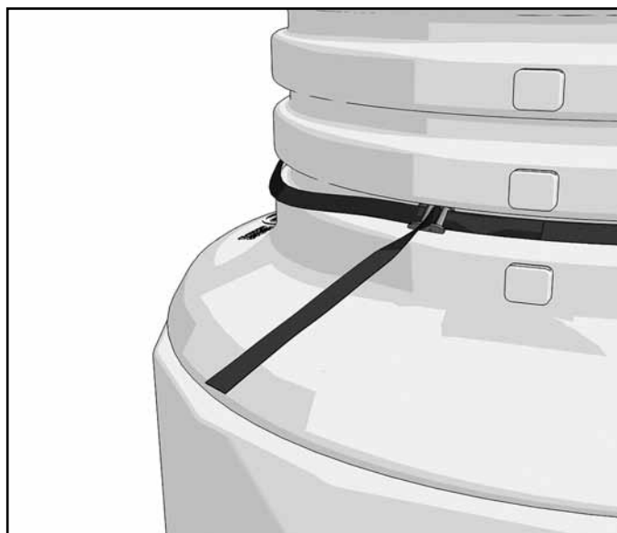
Figure 16: Pull top strap tight with cam buckle
