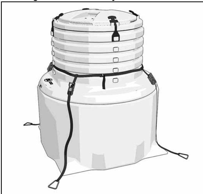
Figure 14: For Deep Burial, pass the harness over the riser and position the top strap above the lower rib.
