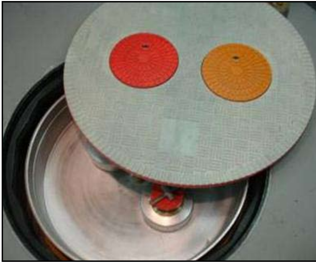
13. Using the FL-7A handle, move the cover into place. Refer to the FL-100 operating instructions.
